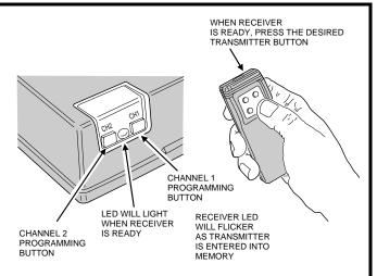
**STEP 6** Add additional transmitters. Repeat Step 5 for each transmitter used with this receiver. Be sure to press the receiver's program button *each time* a new transmitter or a different transmitter button on a multi-button transmitter is pressed.
