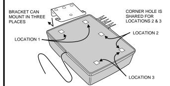
MDR - Single-channel external receiver with relay output.
