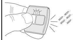
PROGRAM THE TRANSMITTER INTO THE RECEIVER BY PLACING THE RECEIVER INTO PROGRAM MODE. THEN SEND SIGNAL TO THE RECEIVER FROM THE TRANSMITTER. REFER TO THE RECEIVER'S PROGRAMMING INSTRUCTIONS
