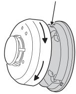
TWIST SMOKE ALARM CLOCKWISE TO LOCK ONTO MOUNTING PLATE
