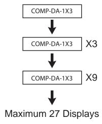
Maximum recommended distance of component cabling between each COMP-DA-1X3 or display (1080p) is 50 ft. Maximum number of displays that are supported in a large 1x3 Component / Audio DA system is 27.
