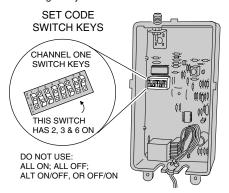
STEP 5 Connect receiver to power. Connect the red power input wire to the 24VDC radio power and the black wire to the common terminal on the gate operator. Alternately connect wires to a 12-24 VAC transformer.
