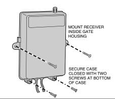
STEP 7 Connect antenna. Connect the coaxial cable to the "F" connector on the receiver. Drill a 3/8" hole on the top of the operator housing for the bulkhead connector. Insert the connector and secure it with the nut and lock washer. Connect the cable and antenna to the bulkhead connector.
