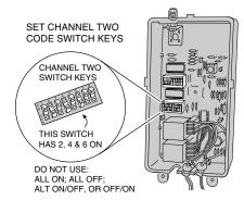
the coding switch on the transmitter and set the eight keys identical to those on the desired channel of the receiver. Be sure they match exactly. If using a two or four-channel transmitter, refer to the coding instructions included with the transmitter for proper system codina.
