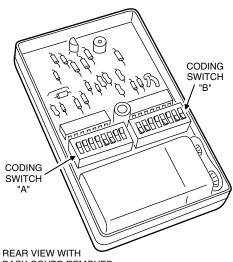
BACK COVER REMOVED TO ACCESS SWITCH "B"
