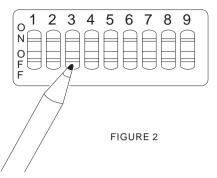
To gain access to the switch, remove the top section of the cabinet, if you have not already done so, Using a pencil, or other similar device, move the code switches to set your house code. Positions one through nine on most MULTI-CODE transmitters are used to set the house code. NOTE: THE MULTI CODE 4120 TWO CHANNEL TRANSMITTER OR 4140 FOUR CHANNEL TRANSMITTER REQUIRES A DIF-FERENT CODE SELECTION. REFER TO THE APPROPRIATE INSTRUCTIONS IF THERE IS ANY DOUBT AS TO CORRECT SETTING.
