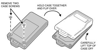
REPLACE THE REMOTE CONTROL BATTERIES WHEN THE UNIT ONLY WORKS CLOSE TO THE CONSOLE OR IF IT STOPS WORKING ALTOGETHER
