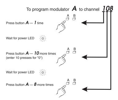
If an error has occurred, the LED will flash quickly for a second and return to the previous settings. On Model 3025, if two adjacent channels are selected, the unit will accept the entry but the LED will blink continuously.
