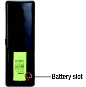
Figure 3-3: Battery pack installed
