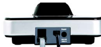
Figure 3-1: Telephone cable connection
