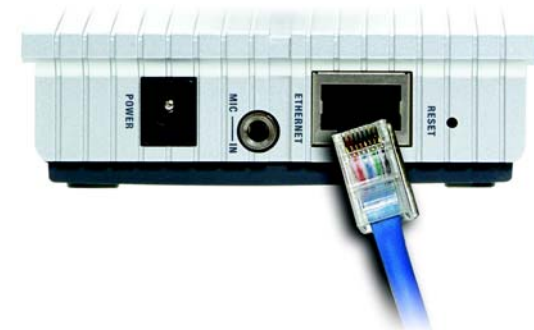
Figure 4-1: Connect the Ethernet Network Cable
