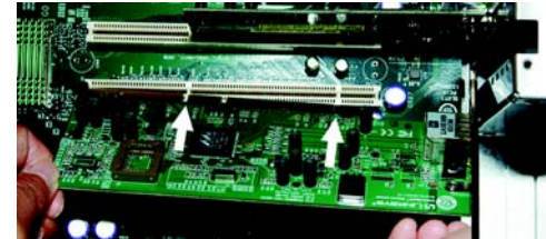
Figure 3-1: Insert the Adapter into the PCI Slot
