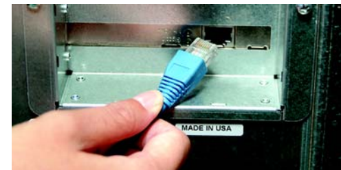
Figure 3-3: Connect the Ethernet Network Cable
