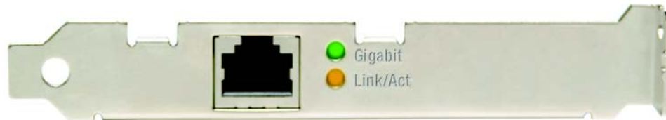
Figure 2-1: Port and LEDs
