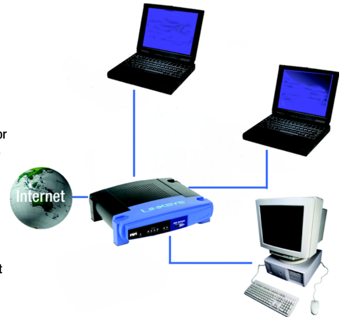
Figure 2-1: A Network with the Gateway
