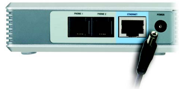
Figure 3-4: Connect the Power
