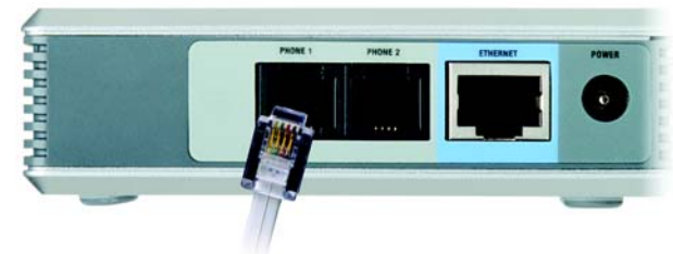
Figure 3-2: Connect the RJ-11 Telephone Cable
