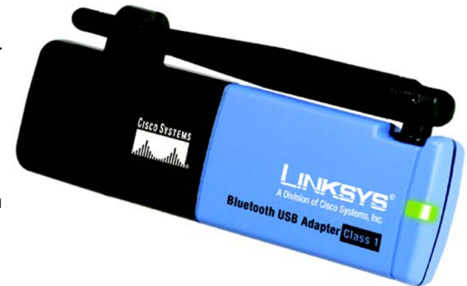
Figure 1-1: The Bluetooth USB Adapter
