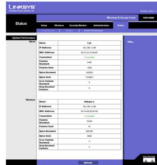
Figure 6-26: Status - System Performance
