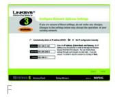
**SSID**. The SSID is the unique name shared among all points in a wireless network. The SSID must be identical for all points in the wireless network. It is case sensitive and must not exceed 32 characters, which may be any keyboard character. Make sure this setting is the same for all points in your wireless network.
