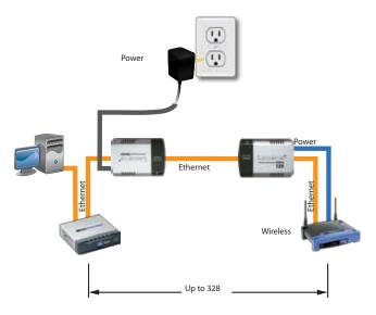
To connect the Kit to a device with a conventional power port, proceed to the section, "Power on a Device that Uses a Standard Power Adapter." To connect the Injector to a device that supports inline power, proceed to the section, "Power on a Device that Uses Inline Power."
