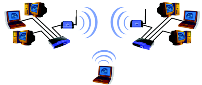
Figure 2-3: Wireless Bridging Using Two Bridges
