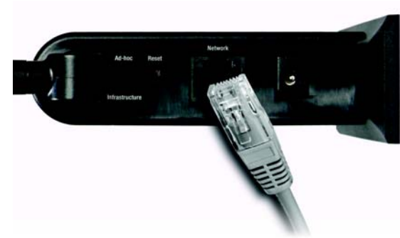
Figure 4-1: Connect the Ethernet Network Cable
