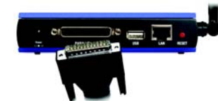
Figure 3-3: Connecting to the Parallel Port
