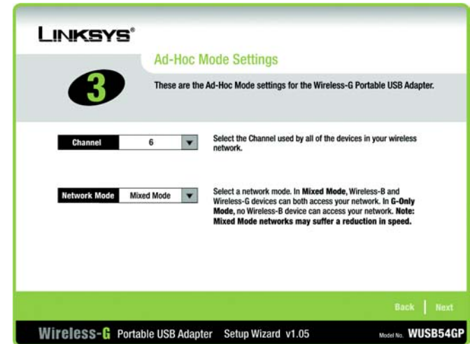
Figure 3-4: The Ad-Hoc Mode Settings Screen
