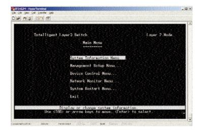
The Main Menu screen consists of a series of options. Each option leads you to the screen for that management setting. Highlighting any option selects it; pressing the **Enter** key takes you to that screen.
