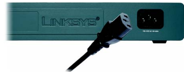
Figure 4-5: Connect the Power
