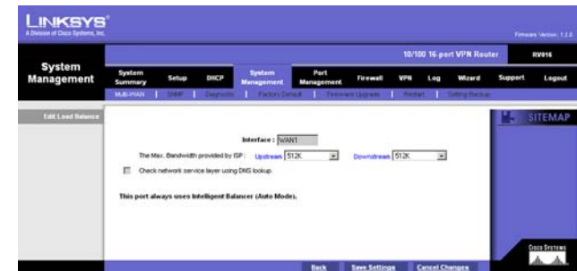
Figure 6-30: Intelligent Balancer - Edit Load Balance
