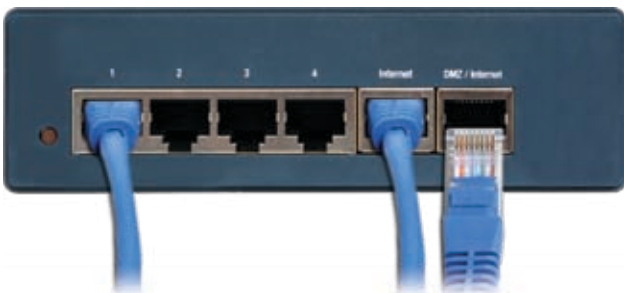
Connect to the DMZ/Internet Port
