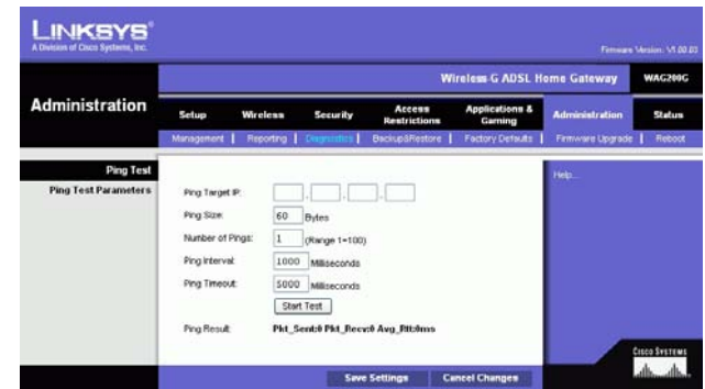
Figure 5-36 : Ping Test (Test Ping)
