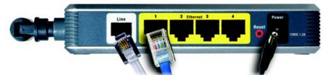
Figure 4-5: Connect the Power
