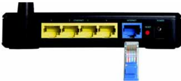
Figure 4-5: Connecting Another Router
