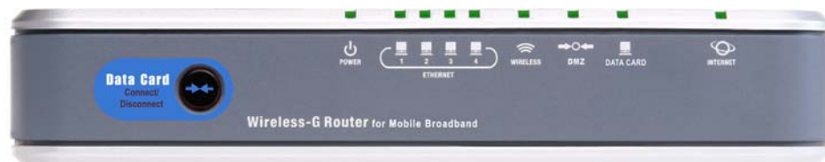
Figure 3-3: The Router's LEDs
