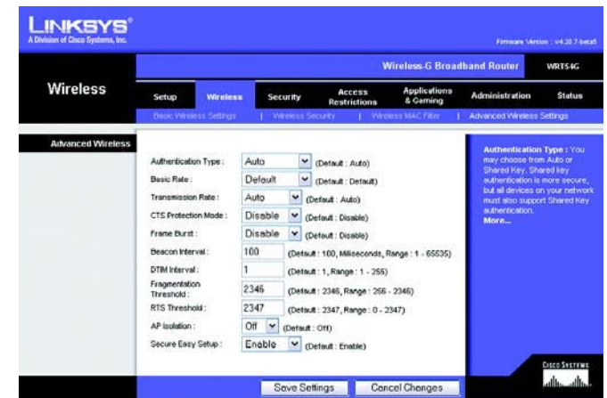
Figure 5-26: Wireless Tab - Advanced Wireless Settings
