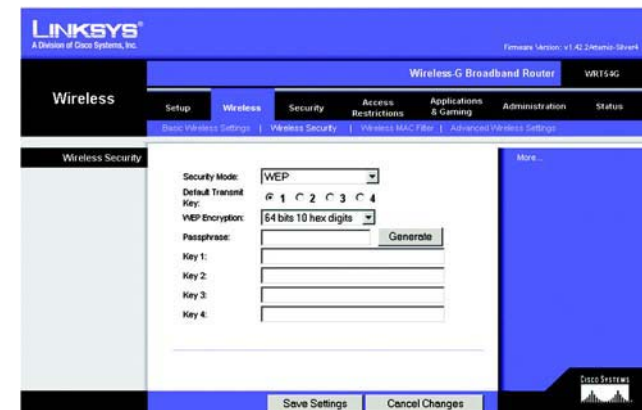
Figur 5-23: Fanen Wireless - Wireless Security (WEP) (Trådløs - Trådløs sikkerhed (WEP))
