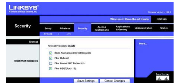
Figur 5-27: Fanen Security - Firewall (Sikkerhed - Firewall)
