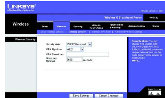
Figuur 5-20: Tabblad Wireless (Draadloos) - Wireless Security (WLAN-beveiliging) (WPA2 Personal)
