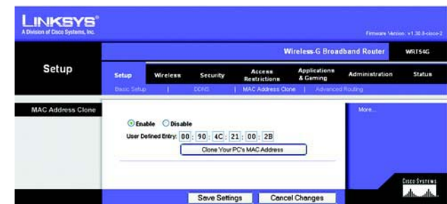
Figure 5-14: Setup Tab - MAC Address Clone
