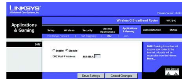
Figure 5-36: Applications and Gaming Tab - DMZ
