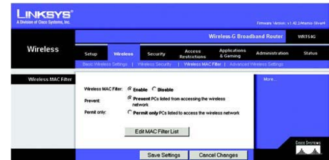
Figure 5-24 : Onglet Wireless - Wireless MAC Filter (Sans fil - Filtre MAC sans fil)
