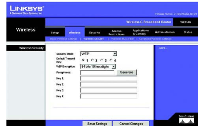
Abbildung 5-23: Registerkarte „Wireless“ – „Wireless Security (WEP)“ (Wireless-Sicherheit (WEP))
