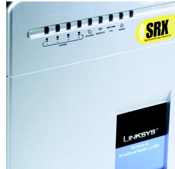
Figure 3-3: The Router's LEDs
