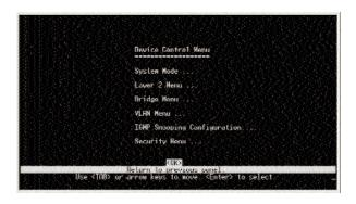
**Note:** This screen shot shows the Device Control Menu displayed by a Layer 2 switch.
