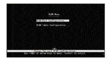
• VLAN Port Configuration - Configures GARP, the default VLAN identifier, default port priority, VLAN tagging on the attached link, GVRP and
