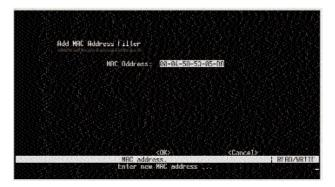
MAC Address - The MAC address of a host device attached to this Switch.
