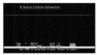
To add an IP address, use **Add**. To delete an address, highlight it with the cursor and press **Enter**. Select **Apply** to make changes. Select **OK** to return to the previous panel. Select **Prev Page** to view the previous page. Select **Next Page** to view the next page. To display a specific page, set the page number in the Page field and then press **Apply**.
