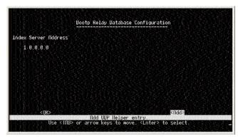
• Index Server Address - Used to define any preferred DHCP servers or the outbound subnetwork for relaying a DHCP request broadcast. (Up to five entries are permitted.)
