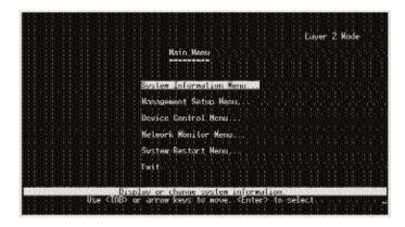
The Main Menu screen consists of a series of options. Each option leads you to the screen for that management setting. Highlighting any option selects it; pressing the **Enter** key takes you to that screen.
