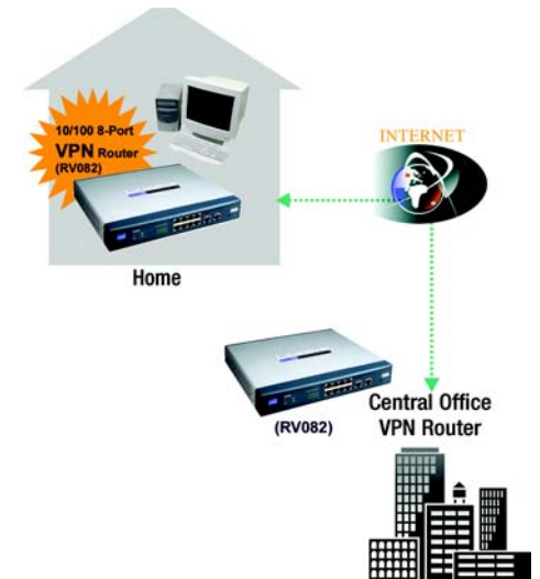
Figure 2-1: VPN Router-to-VPN Router VPN
