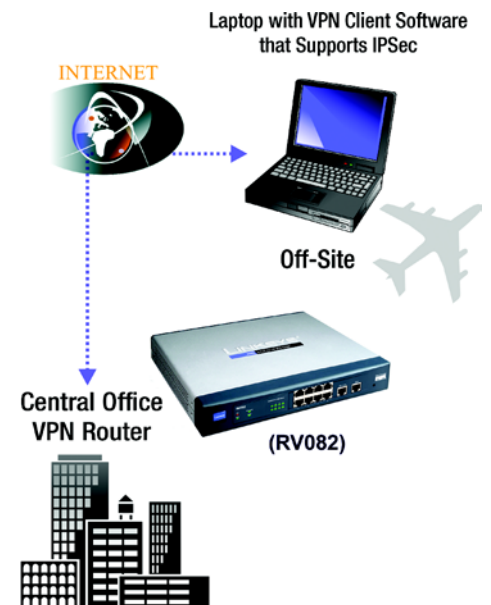
Figure 2-2: Computer-to-VPN Router VPN
