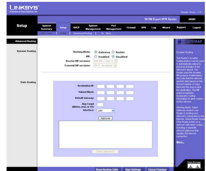
Figure 5-21: Setup Tab - Advanced Routing
