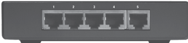
Back Panel of the 5-Port Switch
