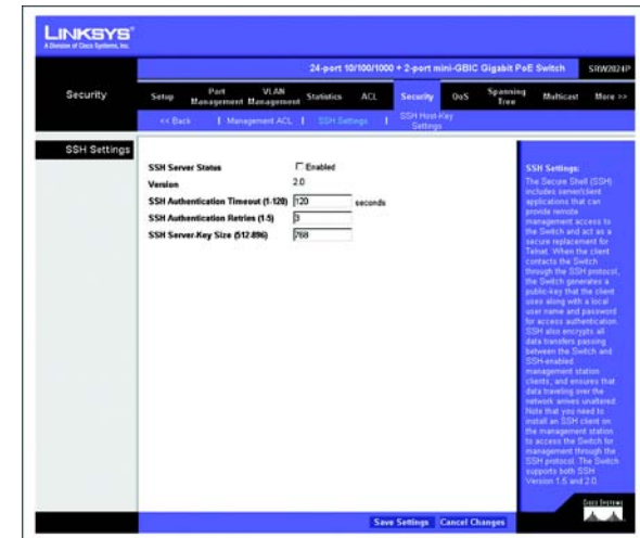
Figure 5-33: Security - SSH Settings
