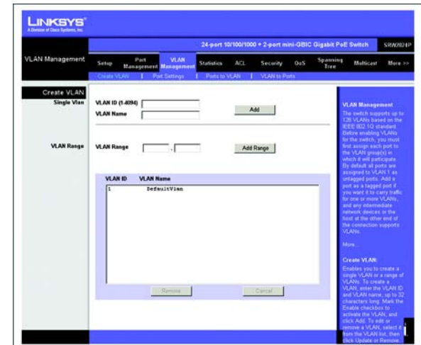
Figure 5-12: VLAN Management - Create VLAN
