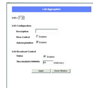
Figure 5-9: Link Aggregation - Link Aggregation Detail
