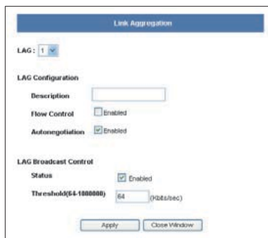
Port Management > Link Aggregation > Detail
