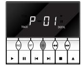
Press DIS (DISPLAY) to save this programme step. Using SKIP or the handset repeat for all chosen tracks then press PLAY.
