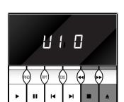
User Options. To customise the operation of the IKEMI and GENKI go to the User Options mode. Switch the power on while holding the **OPEN** button for twelve seconds. **OPEN** selects the Option, **STOP** changes its value. See the following table for the options. To exit press and hold **OPEN** for five seconds.
