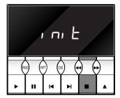
Factory default settings (initialise). Switch the power on while holding the **STOP** button, for ten seconds.
