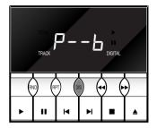
Load a disc and press **OPEN**. Wait until the display shows the disc time then the number of tracks. Press and hold **DIS (DISPLAY)** for two seconds. To start again press **OPEN**.
