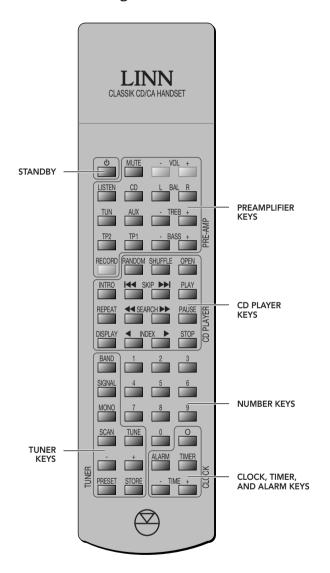
The IKEMI and GENKI are supplied with a remote control handset which provides access to all of the functions available from the front panel. In addition it provides several more advanced features, including selecting tracks by number and programming a selection of tracks.
