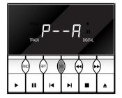
Load a disc and press OPEN. Wait until the display shows the disc time then the number of tracks. Press and hold DIS (DISPLAY) for one second. Holding for longer will enter programme mode B. To start again press **OPEN**.
