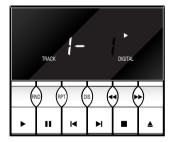
To select a two digit track number press the first digit and hold for two seconds.
