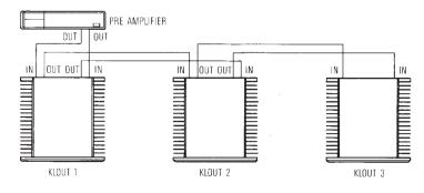
**<u>CAUTION</u>** When passively bi-amping or tri-amping loudspeakers remove any connecting links that are at the speaker input terminals. Failure to do this will short the amplifier outputs together and may damage the power amplifier.
