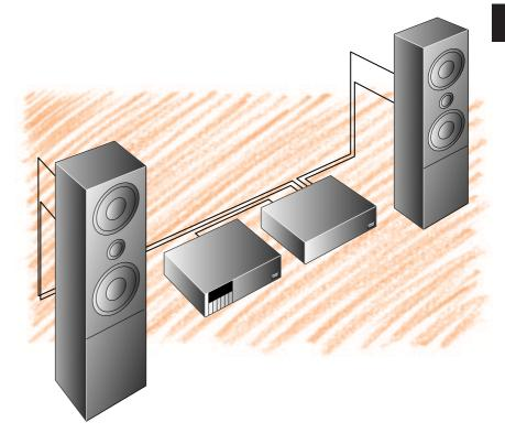
For more performance, you can use two or three LK85/140s to bi-amp or tri-amp to the loudspeakers, each amplifier driving the bass, midrange, and treble signals separately.
