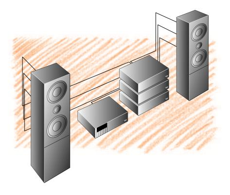
When bi-amping or tri-amping the highest possible performance can be obtained by removing the passive crossover units from the loudspeaker and fitting active crossover modules to the LK85/140 to accurately divide the signal into the appropriate frequency bands. This is known as active playback.
