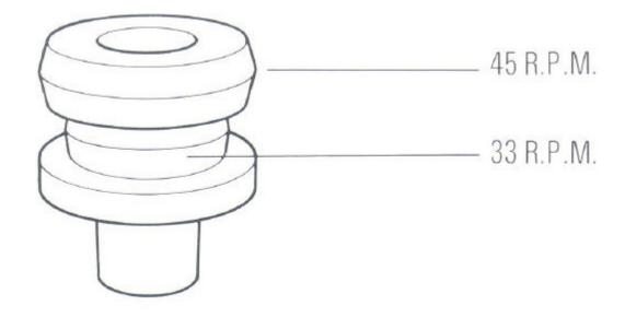
If changing to 45rpm it is advisable to start up the motor with only the inner platter in place, to allow the belt to find a stable position.
