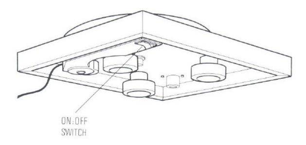
Lift and lower the lid carefully as it is coupled to the suspended plinth. If dropped or roughly handled it may cause the arm to jump.
