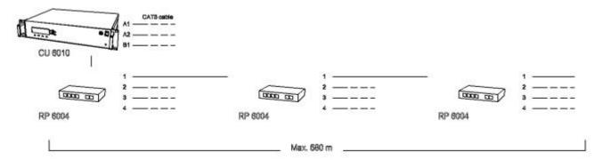
When connecting the RP 6004 Repeaters to the CU 6010 the first RP 6004 is connected to the 'Loop through' connector. The next RP 6004 Repeaters can be connected to either the other 'Loop through' connector or to one of the 'Repeated out' connectors. If using the 'Repeated' outputs
