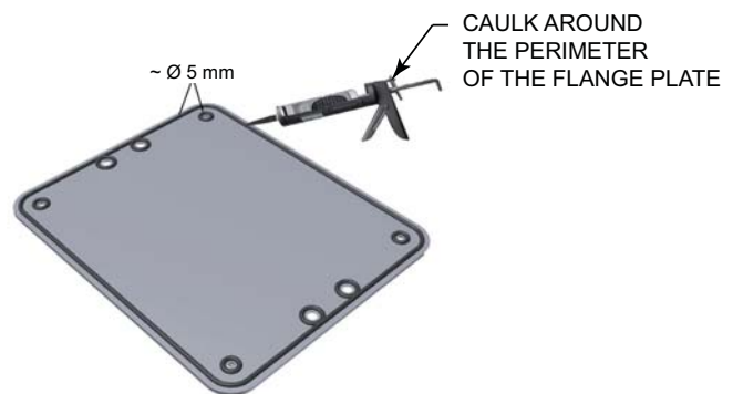
Figure 3-26 Caulk Around Perimeter of Flange Plate
