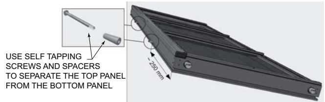
Figure 4-9 For Stacked Series Installations - Use Self Tapping Screws and Spacers
