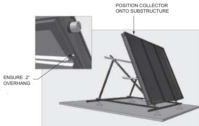
Figure 4-26 Position Collector On Substructure
