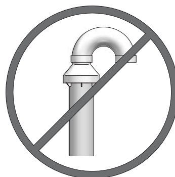
Figure 5-5 Do Not Install U-Bend to Rain Cap
