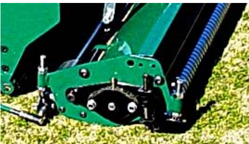
Front and Rear Rollers are infinitely adjustable.
