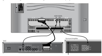
Connect the output socket of the DVD player (DIG OUT) to the TV's "AUDIO DIGITAL IN" socket with a cinch cable.
