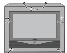
leave at least 5 cm at the sides and 10 cm at the top to ensure sufficient air circulation.
