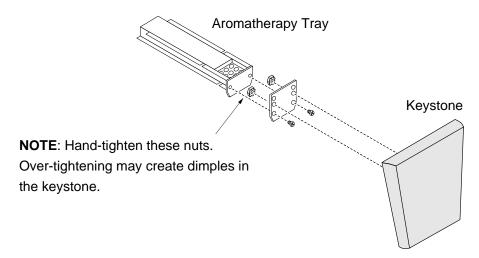
3 Attach the extension assembly to the fireplace following the directions included with the aromatherapy kit.
