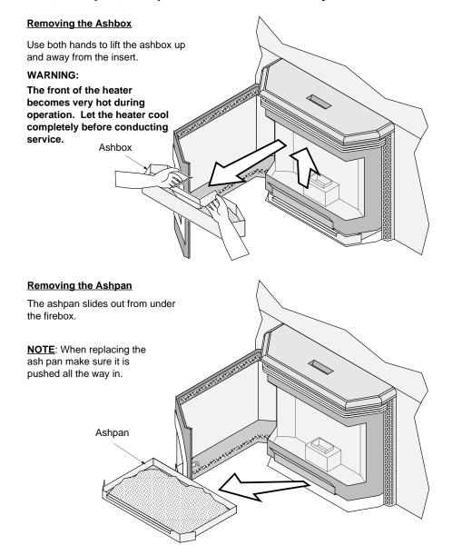
Disposal of Ashes – Ashes should be placed in a metal container with a tight fitting lid. The closed container of ashes should be placed on a non-combustible floor or on the ground, well away from all combustible materials, pending final disposal. If the ashes are disposed of by burial in soil or otherwise locally dispersed, they should be retained in the closed container until all cinders have been thoroughly cooled.
