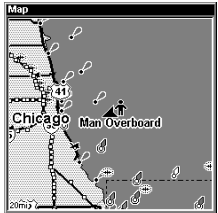
Navigating to Man Overboard: Navigation Page, left, and Map Page, right. The victim is astern of the vessel; the GPS shows which direction to steer to for the rescue.
