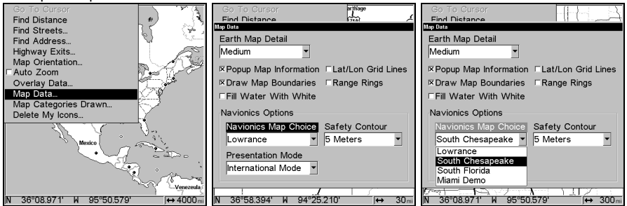
These figures show menu sequence (from left to right) for selecting a Navionics chart for the South Chesapeake Bay area.
