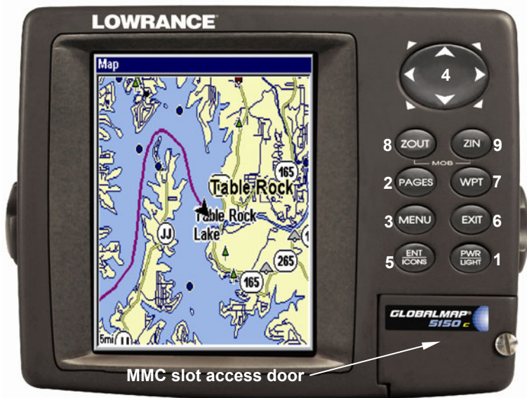
GlobalMap 5150c GPS unit, front view, showing Map Page, keyboard and access door for the MMC slot.
